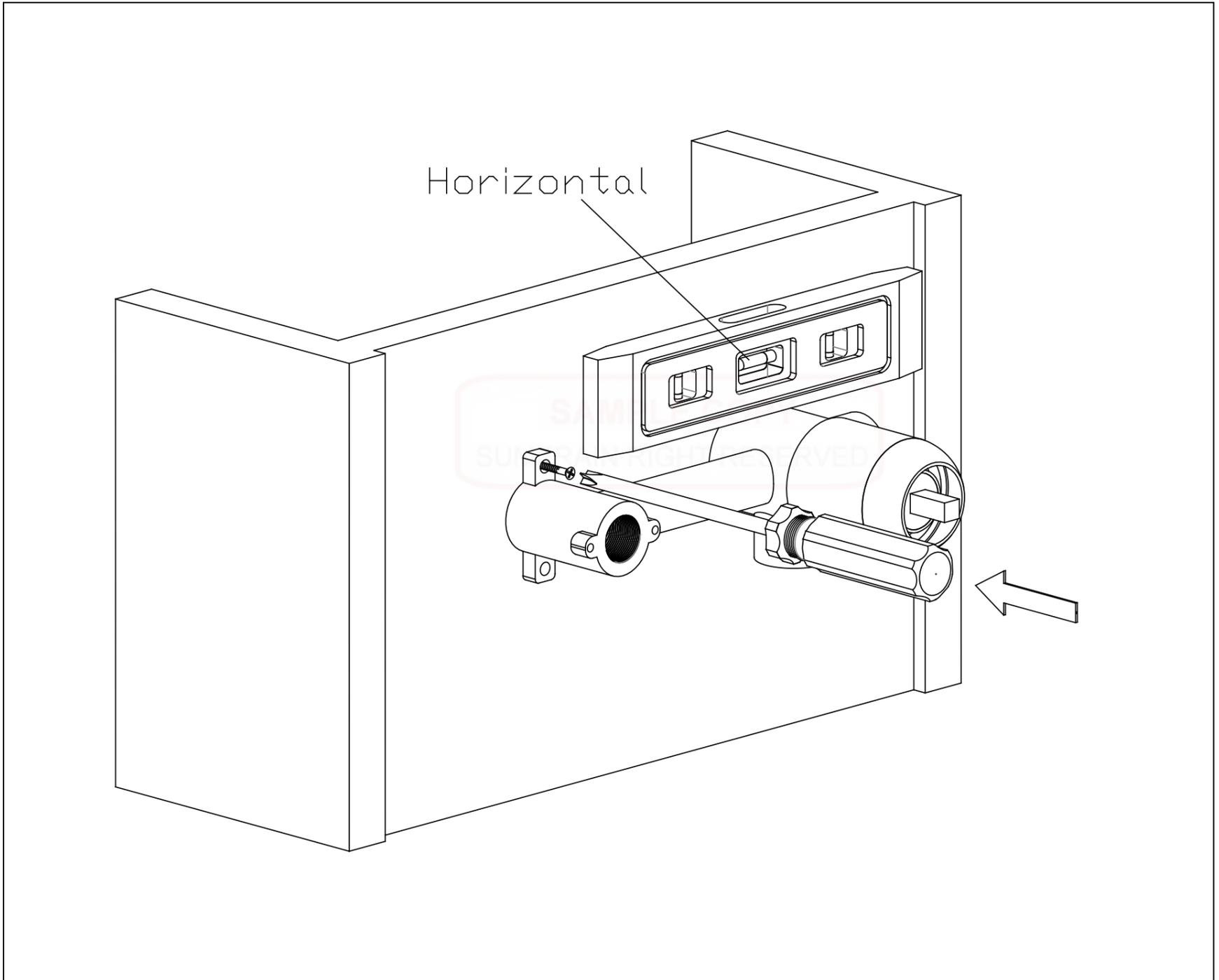
4.3 Turn on your shut-off valve for cleaning the hot and cold water supply tube before connect to the valve trim, allow the water flush 3~5 minutes to flush out dirt and debris. Shut off the water supply again after finish.
