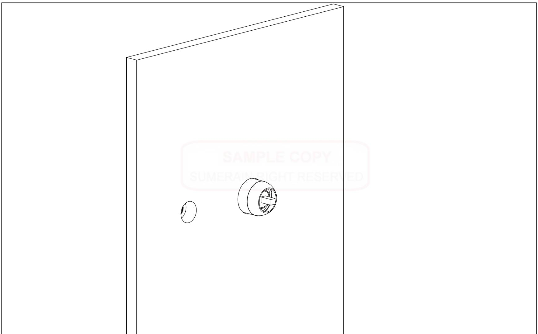
4.6 Apply Teflon tape on the thread of nipple and then connect to rough-in valve
