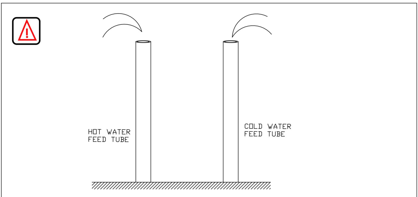
4.4 Apply Teflon tape on the thread of supply tube outlet and then connect to rough-in valve with elbow.
