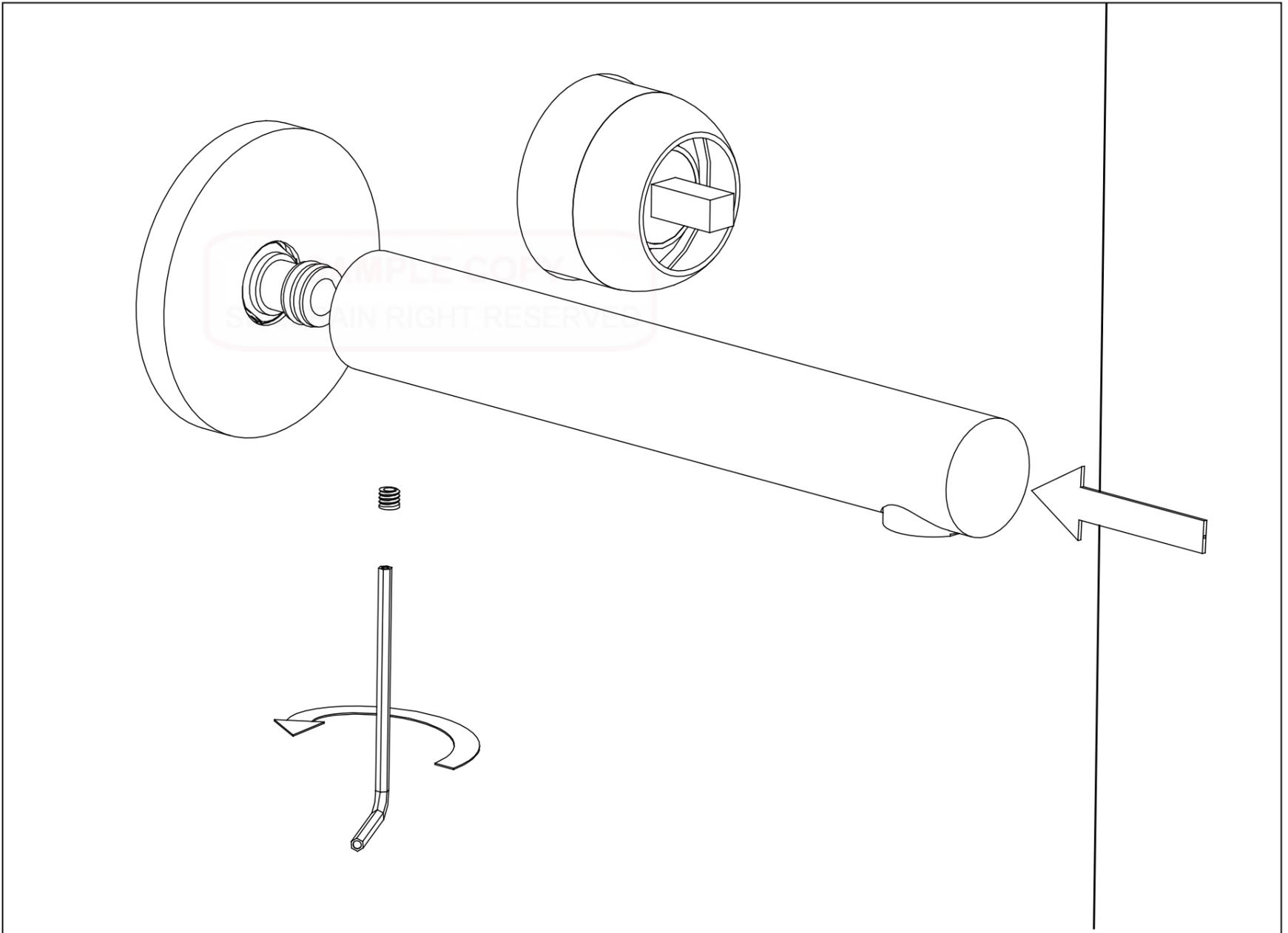
4.9 Slide the escutcheon over the sleeve and attached to the finished wall
