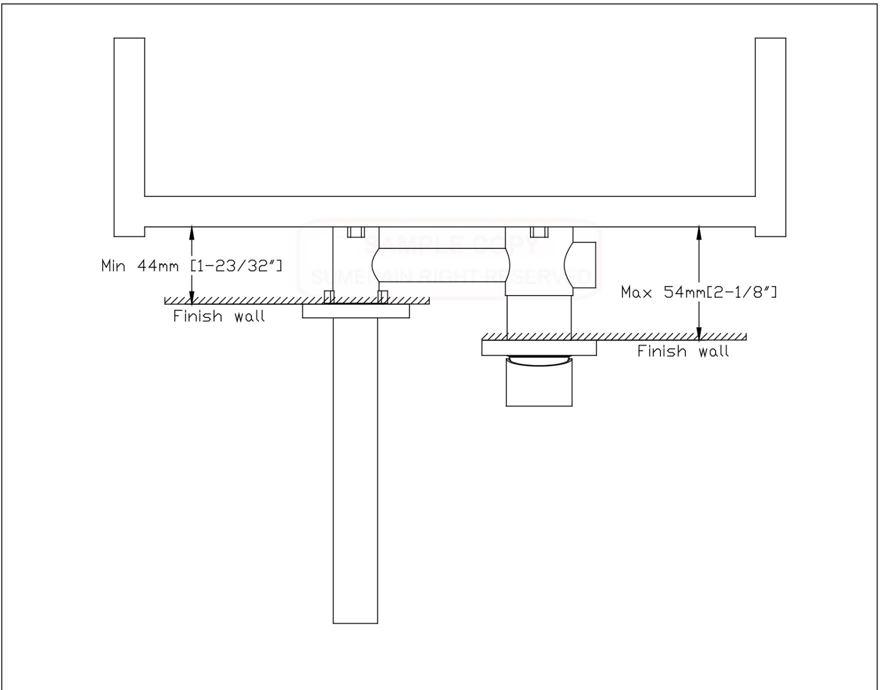
4.2 Secure the rough-in valve to the mounting rack with screws (screws not including)
